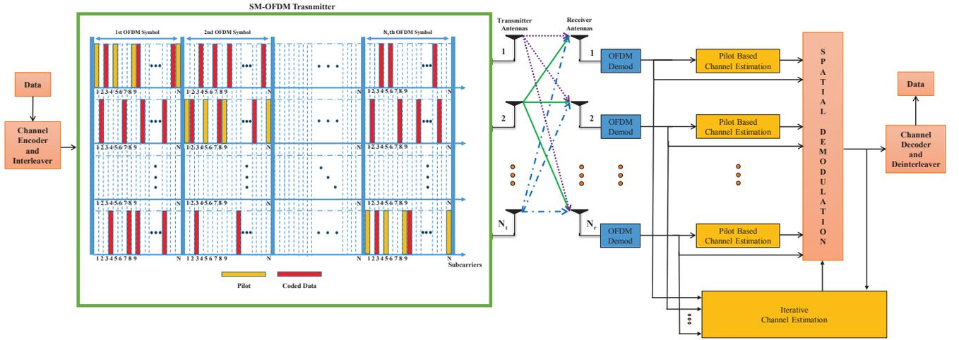
Fig. 2: Block diagram and frame structure of SM-OFDM system
