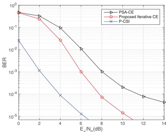
Fig. 4: The BER performance of  $4 \times 4$  coded BPSK-SM-OFDM with channel estimation under TU channel model
