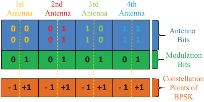
Fig. 1: SM-OFDM mapping table structure
