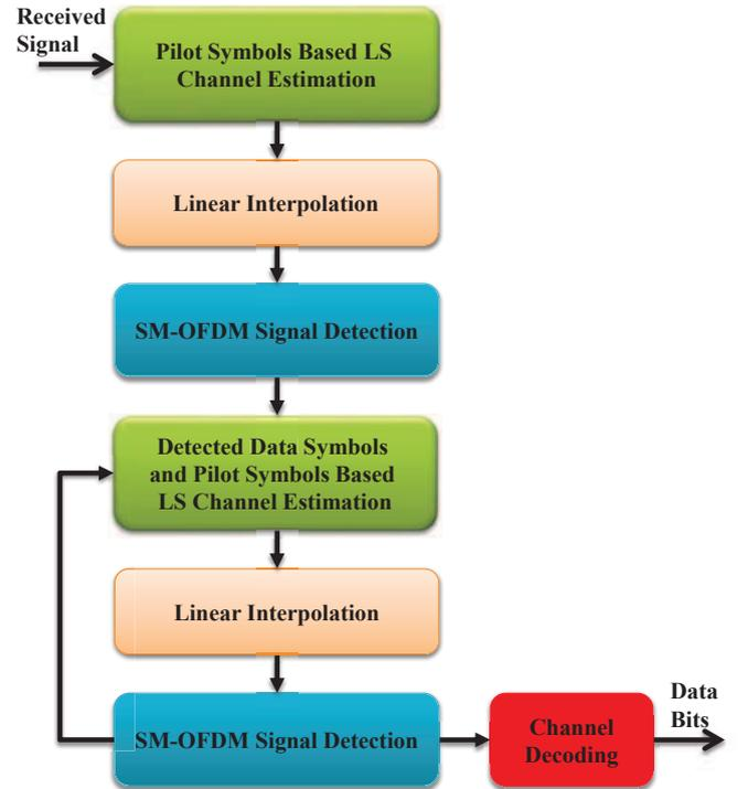
Fig. 3: Block diagram of proposed iterative receiver
